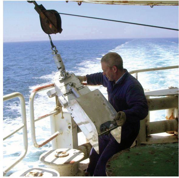
Deploying the Continuous Plankton Recorder from the ship "Pride of Bilbao" Photo: David Johns, SAHFOS.
